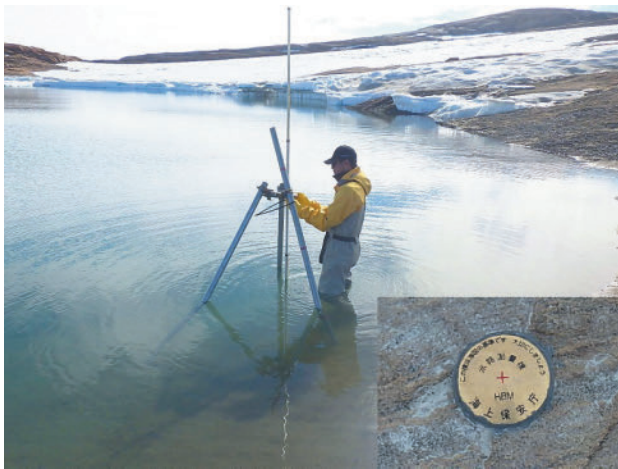
Photo 7. Tide level monitoring equipment and HBM (bottom right) in Rundvagshetta.
