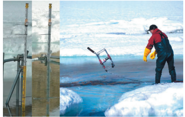
Photo 6. Automatically photographed leveling staff at low tide (left) and high tide (center) and installation of tide gauge in Langhovde.
