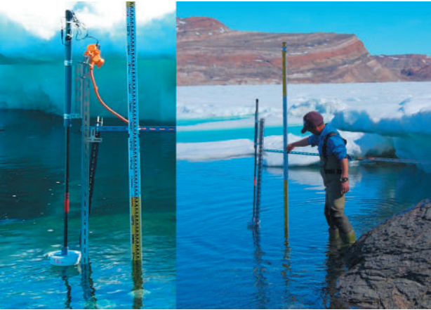
Photo 4. Digital tide level monitoring system (left) and tide level monitoring equipment in Skallen (right).
