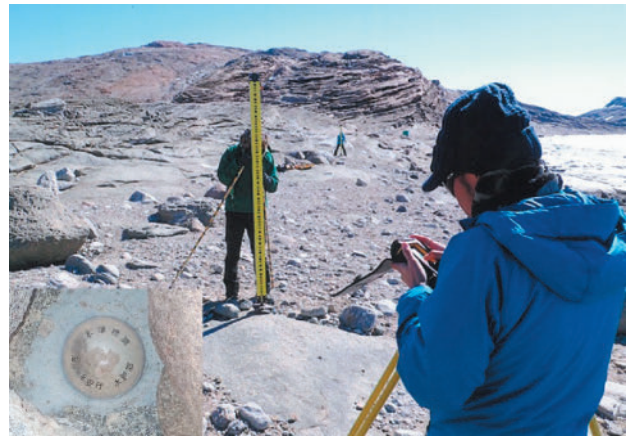
Photo 3. Level survey and Hydrographic survey Bench Mark (HBM; bottom left) in Skarvsnes.
