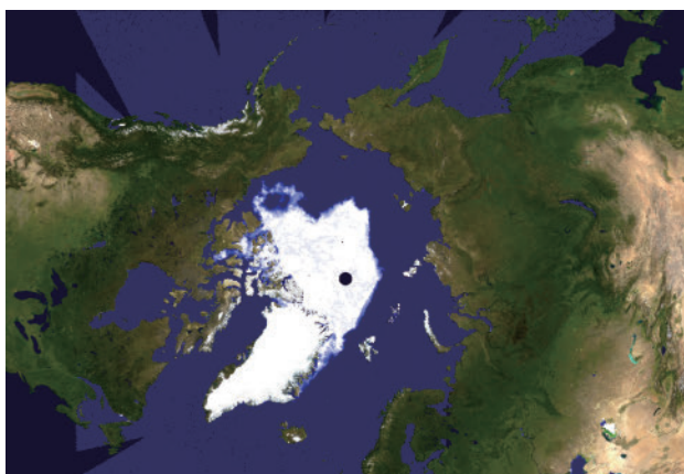
Fig. 7. MSIL is capable of showing sea ice information in the Arctic Ocean. This figure is an example of an image with sea ice concentration information in the Arctic region. The center of the image is Arctic Ocean, the upper part is Pacific Ocean and the lower part is Atlantic Ocean. The white part shows the sea area covered with ice (ice concentration area). The black point is the part that has no data as it is out of satellites orbit.
