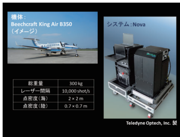
Fig. 3. System overview of Nova.
