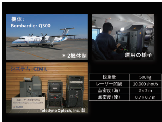
Fig. 2. System overview and major specifications of CZMIL.
