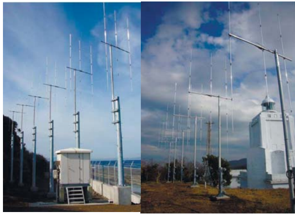
HF radar stations for Sagami Bay area (Left: Ara Saki station, right: O shima station)
