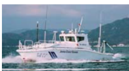
JINBEI Gross Tonnage: 5t (JHOD Hqs) Length 11.0 meters
