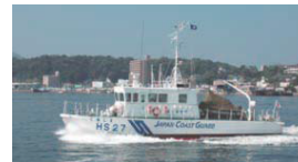
KURUSHIMA Gross Tonnage: 27t (6th RCGHqs) Length 20 meters
