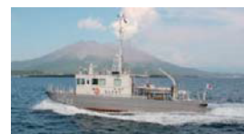
ISOSHIO Gross Tonnage: 27t (10th RCGHqs) Length 21 meters
