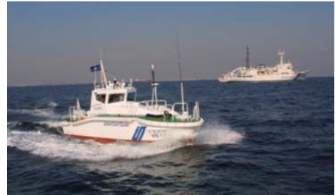
Autonomous survey boat "Jinbei" When a submarine volcano becomes active, surveys of detailed seafloor topography, discolored water, water temperature and so on are safely conducted using "Jinbei" and "Manbo II" equipped with sophisticated survey instruments.
