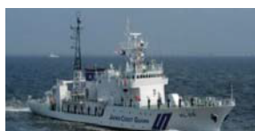
KAIYO Gross Tonnage: 550 t (JHOD Hqs) Length 60.0 meters
