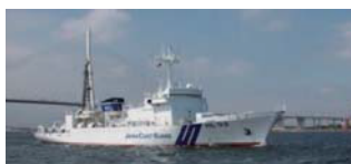
TAKUYO Gross Tonnage: 2,400 t (JHOD Hqs) Length 96.0 meters
