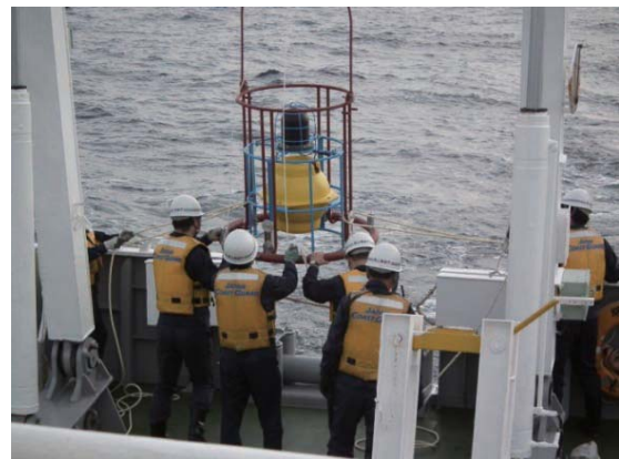
Installing a seafloor station
