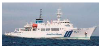
SHOYO Gross Tonnage: 3,000 t (JHOD Hqs) Length 98.0 meters
