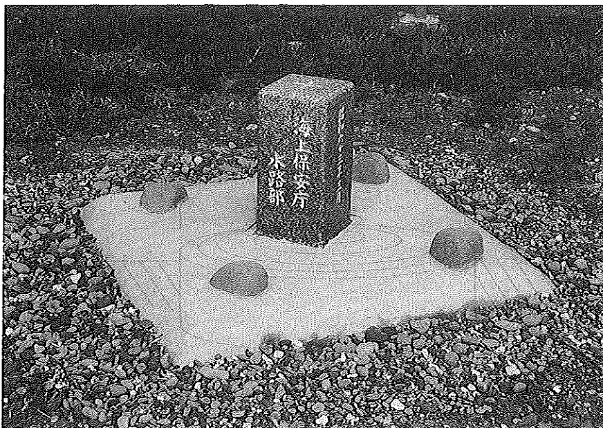
Photo 9. Stone marker for the first order control points.
