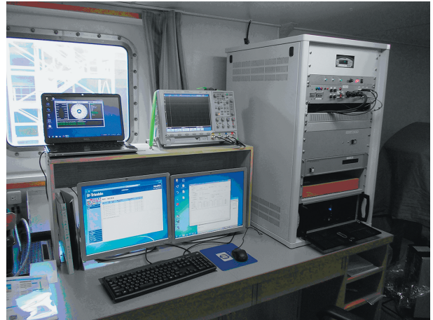
Photo 4. Control and recording devices of seafloor geodetic observation system installed in the S/V Shoyo .
