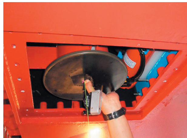
Photo 1. Installation of an acoustic transducer on the hull of the S/V Shoyo.
