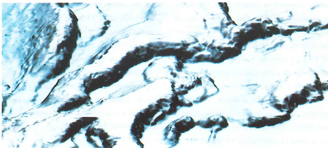
Fig. 7 Improved three-dimensional seafloor image off Akita by two-dimensional DFT approximate, interpolation in the 520 x 460 mesh size. It took about seven days to complete processing.
