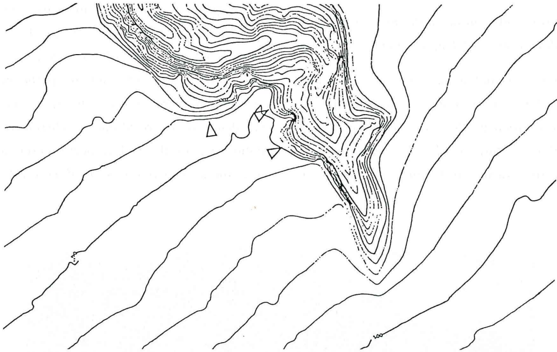
Fig. 2 Contour chart with undesirable artificial topography (marked with \Delta ) was processed by the cubic polynomial approximate interpolation
