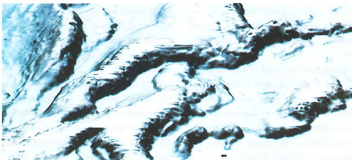
Fig. 6 Unsatisfactory three-dimensional seafloor image off Akita by linear-cubic polynomial approximate interpolation in the 520 x 460 mesh size. It took about 10 minutes to complete processing.
