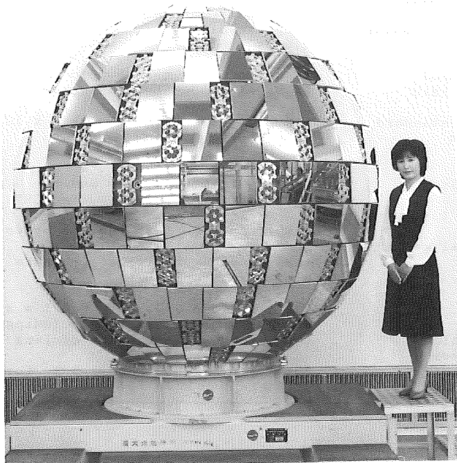
Figure II — 6. Japanese Geodetic Satellite, AJISAI. (215cm of diameter and 1500km of orbital height).
